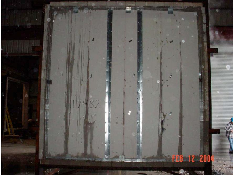
Unexposed face after the hose stream test
