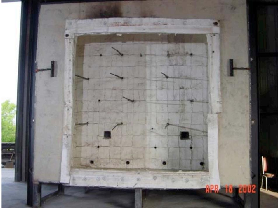
This photograph of the vertical furnace shows it with a concrete adapter in place which reduces its opening to 120" x 120". Without the adapter the furnace will accept test specimens 144" tall x 168" wide. The furnace is 48" deep, with burners on the sides, so that no flame impingement on the specimen occurs.
