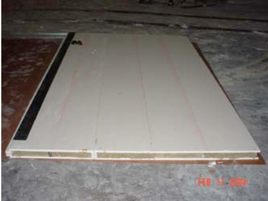
The panels were assembled on the ground prior to mounting in the test frame
