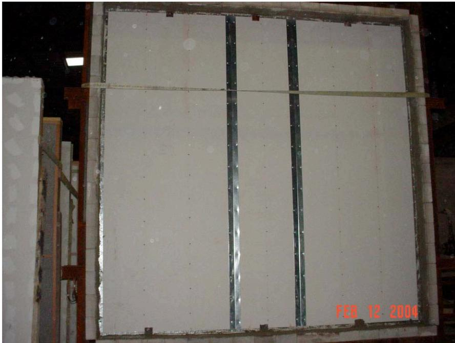
Exposed surface prior to mounting against the furnace
