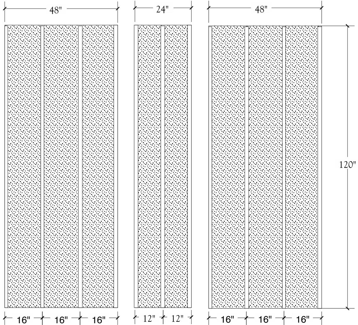
**ELEVATION VIEW** (one side of gypsum removed to show stud details)
