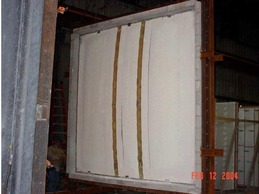
Moving the assembly into position for the hose stream test
