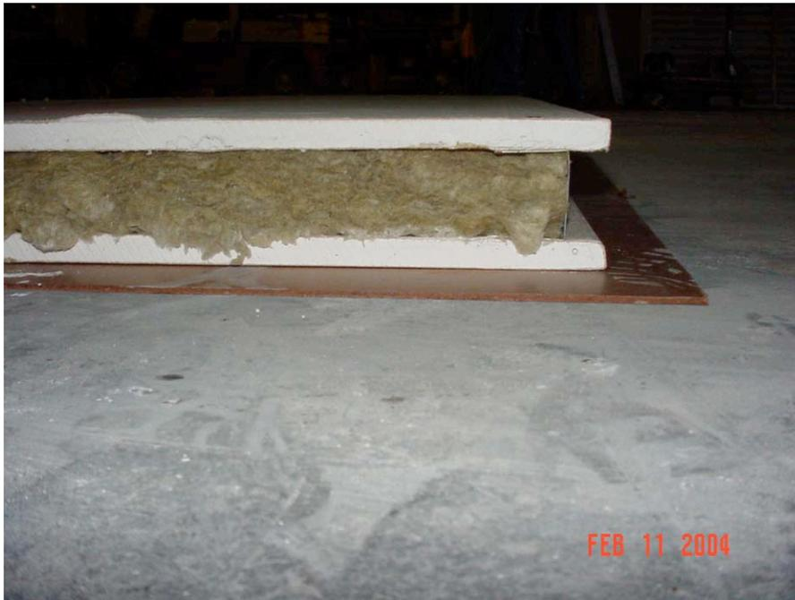
The panel core was insulated with 2" thick Roxul mineral wool
