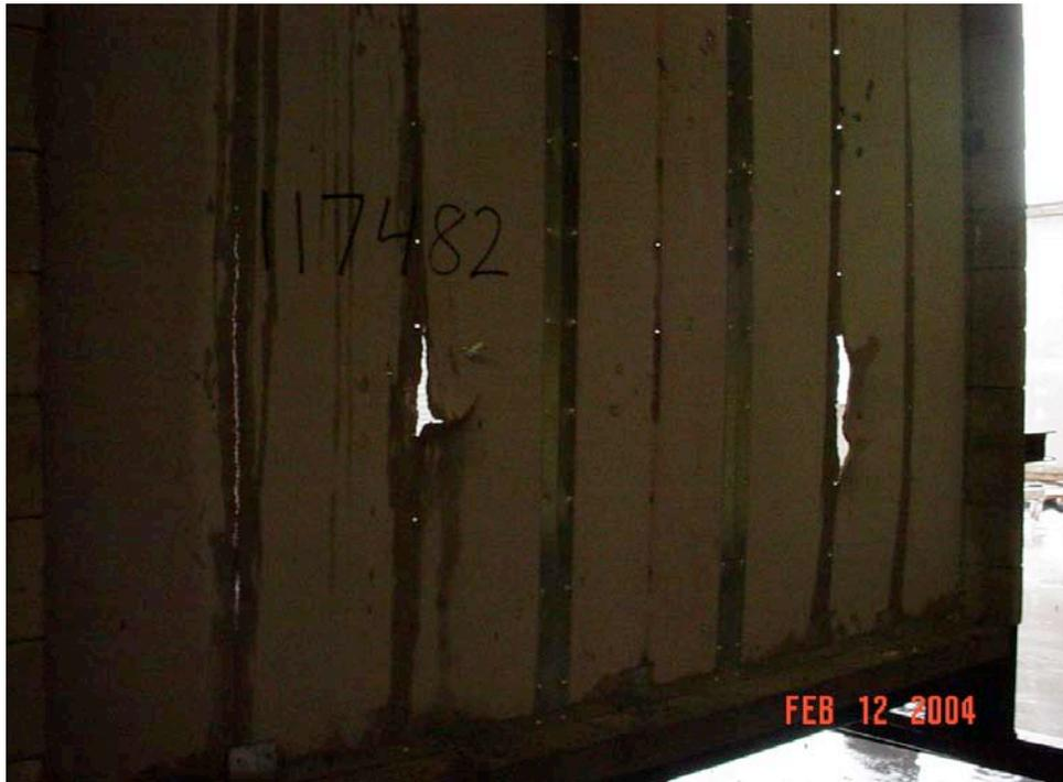
The water stream penetrated the wall in two locations, as shown
