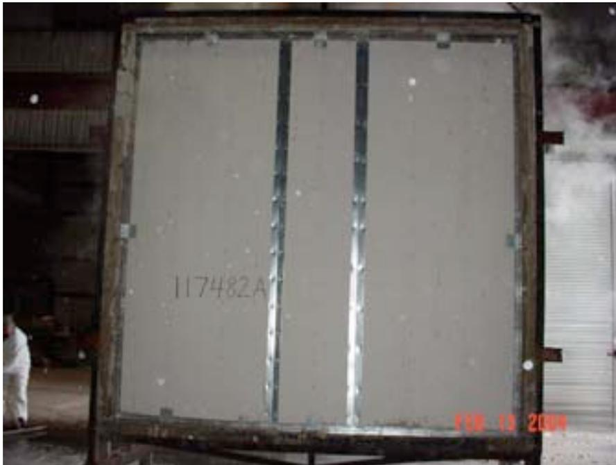
Unexposed face after the hose stream retest
