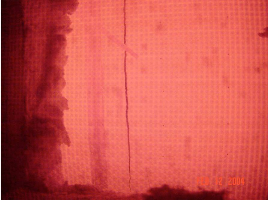
Crack formed in the exposed gypsum wallboard
