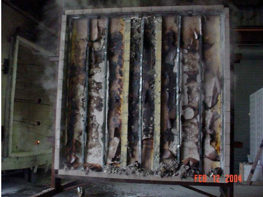
Exposed face after the hose stream test
