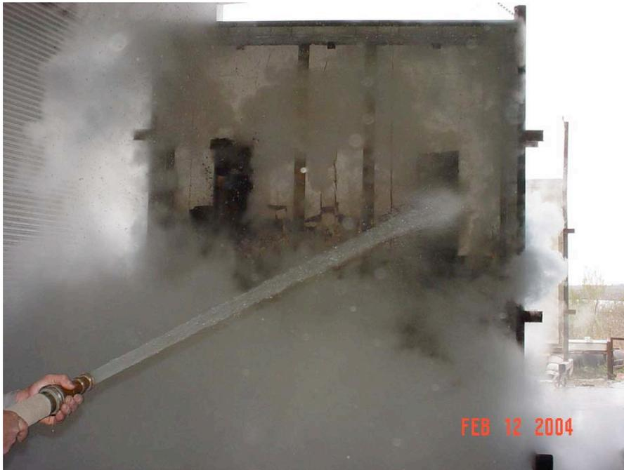
The hose stream penetrated the wall after 48 seconds, indicating a failure
