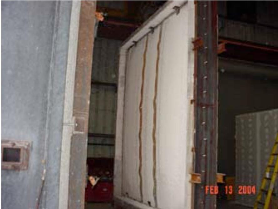
Moving the assembly into position for the hose stream retest
