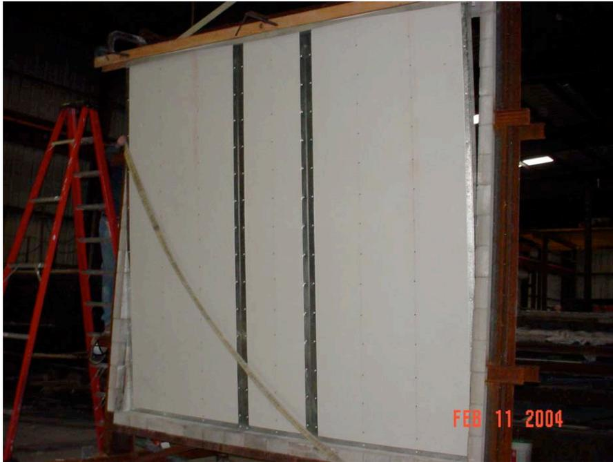
The completed wall was then tipped into place in a nonbearing test frame
