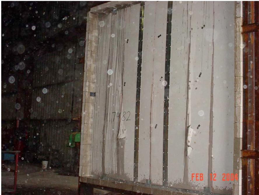
Unexposed face after the hose stream test
