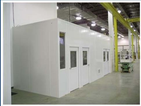
Cleanrooms by Panelbuilt incorporate a hidden return air chase system. Utilizing the wall cavity itself in conjunction with properly sized return louvers, Panelbuilt is able to eliminate the expensive ductwork and/or chase walls often associated with hardwall modular cleanroom systems. This translates into a final product that is more attractive, less expensive, and easier to install.
